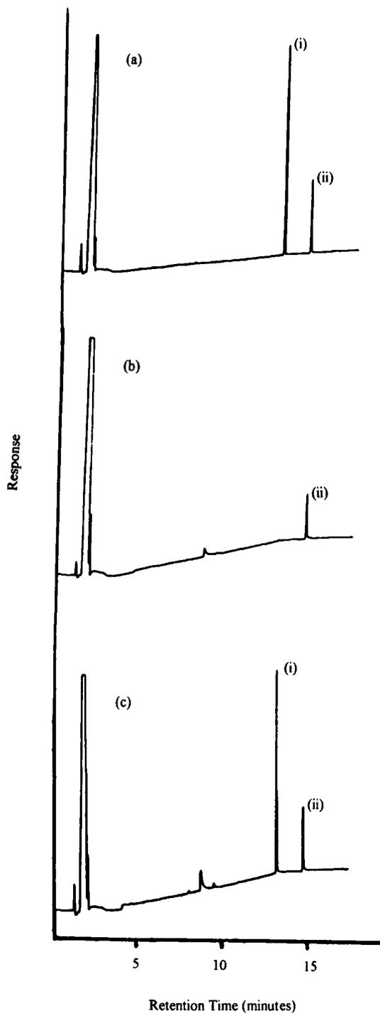
**Figure 3** Gas chromatograms of (a) diazinon standard in hexane (1.0 mg/L), (b) sewage blank, and (c) extraction of 1.0 mg/L of diazinon from a spiked sewage sample. (i) represents the diazinon peak and (ii) the internal standard, fenthion, which was added to each sample (1.0 mg/L).
